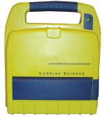
whether a shock is needed. When the operator responds to the prompt to give a shock, an electric current is delivered through the victim's chest wall through adhesive electrode pads.
